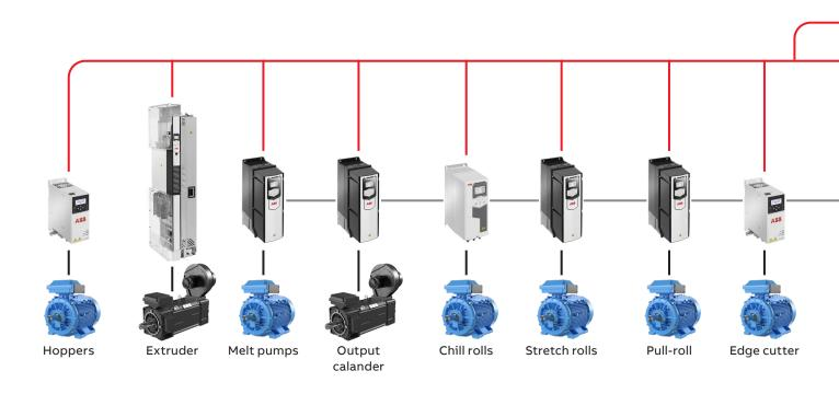
**Connecting the system to cloud-based services** All the ABB motors and drives included in the cast line can be securely connected to ABB Ability<sup>™</sup> cloud services. The connection can be established from our AC500 range of PLCs, or by using third-party PLCs for the gateway to the cloud. The ABB all-compatible drives support all common fieldbus connections.
